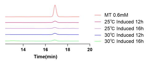
As shown in the figure, strain Bw25113/pSB1c-SgAANAT-CrTDC/pYB1a-AtCOMT\*\*\* can synthesize MT from 5-HTP, but the yield is low. It is speculated that AtCOMT enzyme activity is not high.
